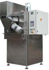
This machine is configured to deflash technical rubber, silicon, plastic and similar productsusing liquid nitrogen.
